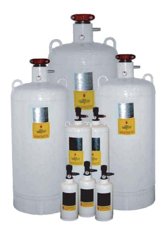
SFM Clean Agent Cylinders are used in fire extinguishing systems to store the Clean Agent unitl a fire develops and the agent must be released. The Clean Agent is retained in the container by a valve assembly which contains a fast acting rupture disc.
