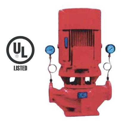
Volute type casing which allows smooth flow. it is made of high quality cast iron with integral square base feet. It is equipped with bronze impeller and stainless steel shaft and sleeves.
